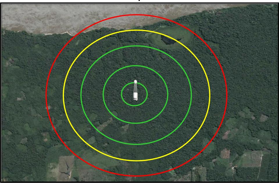
The footprint is defined as the relative contribution at different location (in the upwind direction) to the measured vertical flux
